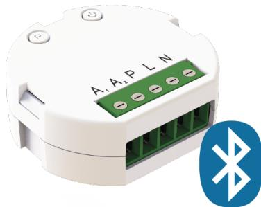
Smart Pill ON-OFF Micro is potential free relays which can be installed in the wall box or similar enclosed installation to turn ON or OFF one or more appliances ex. Electrical panel ovens, garage door motors etc. The device can be controlled with Bluetooth from app, Smart Switch or push switch. You can use them as relay to select either ON/OFF or you have the option to select pulse mode, to give pulse to ex. a motor for a garage door.
