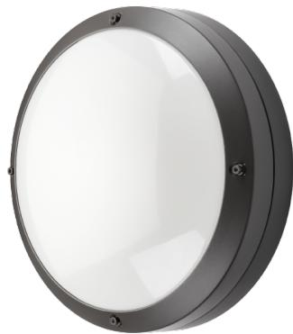
Design: Svein Knudsen / Andrew Smith. Attractive, round luminaire that can be mounted to both walls and ceilings, and both indoors and outdoors. Made of die-cast powder-coated aluminium. Flat diffuser made of UV-stabilised opal polycarbonate. Many variants with both sensors and wireless control, as well as various lumen packages. IP65 and vandal-resistant rating IK10.
