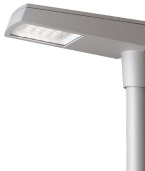
Design: Christian Hvidt. Mast top-mounted LED luminaire. IP66. LED luminaire. Base and top made of die-cast aluminium, front made of tempered glass. Base and diffuser in textured light grey. Direct lens optical solutions (Multilens). Complete with LED driver for operation of LED light sources mounted to component rail with internal connector/lampholder and pre-mounted with six-metre connection cable. Prepared for mounting on 60 mm mast. Safety class II.
