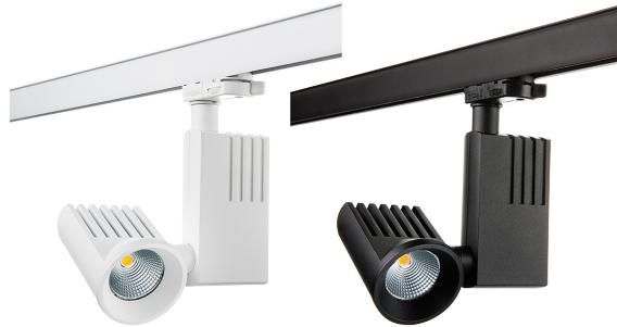
Three-phase rail spot with integrated powerful LED chip and driver. Dimmable with phase dimmer. Mounted using global multi-adapter, which is ideal for SG's three-phase rail system as well as other systems where Global can be used. Perfect colour rendering due to very high RA value and SDCM 2. ZIP Pro Mini is made of powder-coated aluminium, flexible and able to be pointed in almost all directions, making it the obvious choice for all places where spots or effect lighting is to be used.
