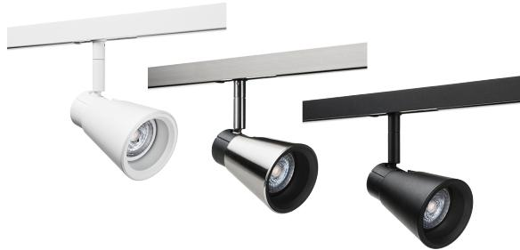
1 circuit rail spot for ZIP rail system with replaceable GU10 LED. Dimmable with phase dimmer.
