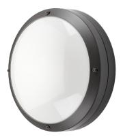
Design: Svein Knudsen / Andrew Smith. Attractive, round luminaire that can be mounted to both walls and ceilings, and both indoors and outdoors. Made of die-cast powder-coated aluminium. Flat diffuser made of UV-stabilised opal polycarbonate. Many variants with both sensors and wireless control, as well as various lumen packages. IP65 and vandal-resistant rating IK10.
