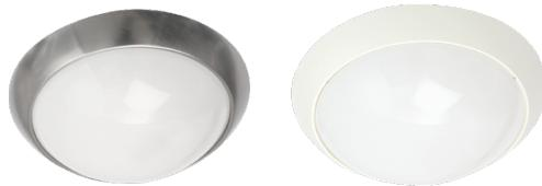
Design: Birger Sevaldson. Round lamp in several sizes. Vandal-resistant with impact-resistant polycarbonate opalescent diffuser. The whole luminaire has been approved for common access routes and has vandal-resistant rating IK10. Kl II, two cable inputs and the option of additional looping using the integrated quick clips. Can be mounted to either the wall or ceiling with both concealed and visible cabling. Many light source variants and sensors, wireless control and emergency light.
