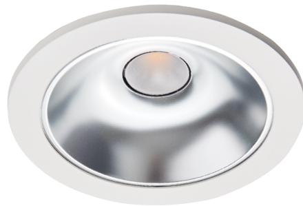
Recessed mounted LED downlight. Made of fire-resistant polycarbonate. SDCM 2. L90/B10>100,000, Supplied with 3000K/4000K LED. Complete with driver and quick connection between driver and downlight for super quick and easy mounting. Can be mounted to ceiling panels with a thickness of 1-50 mm. The luminaire comes complete with ceiling ring RAL9010 gloss 25 made of die-cast aluminium. Matt reflector.
