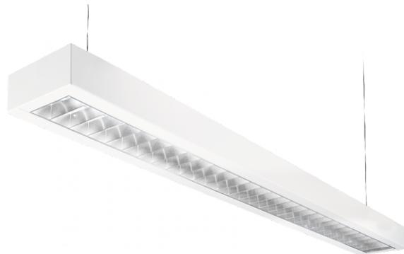
Luminaire suspended/surface-mounted directly in 3000 or 4000 Kelvin LED. Flat design, powder-coated white RAL9010 gloss 25. Double parabolic reflector and diffuser with option of dimmable solution (DALI/SwitchDim). Plug-and-play solution for quick installation. Adjustable wire suspension (2x2 m) ordered as accessory.
