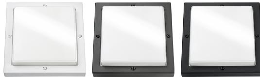
Attractive, square LED wall luminaire that can be installed both indoors and outdoors. Made of die-cast powder-coated aluminium. Diffuser made of UV-stabilised opalescent polycarbonate, two inputs/outputs for cables, option of both visible and hidden cabling, and loopable terminal block. IP65 and vandal-resistant rating IK10.
