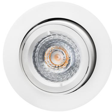
LED downlight for indoor use. Replaceable dimmable GU10 bulb (included). Made of die-cast powder-coated aluminium or brushed steel. Ø83 hole dimensions.
