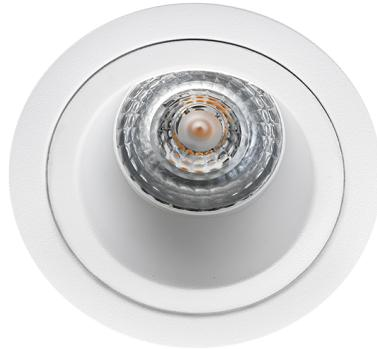
LED downlight for indoor use. Replaceable dimmable GU10 bulb (included). Made of die-cast powder-coated aluminium or brushed steel. Ø83 hole dimensions.
