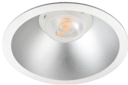
Rax Soft in an asymmetric version for illuminating walls in corridors, offices etc. The asymmetric lens gives excellent light control and provides a conical light pattern on the wall, minimizing glare and giving a comfortable wall illumination. Rax Soft Asymmetric is installed easily with springs that fit ceiling panels with a thickness of 1–50 mm.
