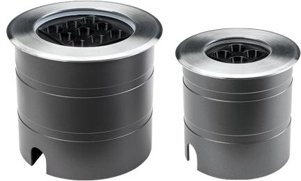
Powerful in-ground luminaires for decorative and functional lighting of facades, gardens, patios, stairs and walls. Approved for 2000 kg load. Nemo II comes in symmetric versions with deep black reflectors for very low glare, and asymmetric versions that directs the light toward a facade or a wall. Nemo Siriak gives a decorative light along patios and facades.
