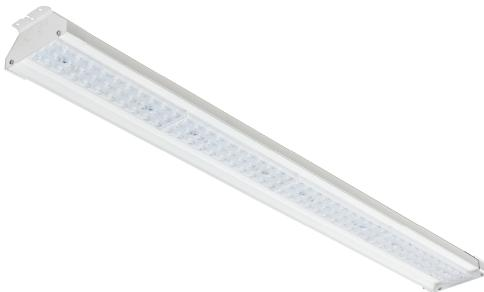
Arena is an energy efficient surface mounted IP23 luminaire for use in industry and storage. It is easy to install with hinged gear tray, and can be mounted either direct on ceiling (screws) or by using the mounting hooks for horizontal wiring. Arena is available in two lengths and with three different light distributions. 5/7-pole terminal block with 5/7x2,5mm<sup>2</sup> through wiring. Cable entry in end caps through grommet.
