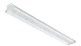
Arena is an energy efficient surface mounted IP23 lumninaire for use in industry and storage. It is easy to install with hinged gear tray, and can be mounted either direct on ceiling (screws) or by using the mounting hooks for horizontal wiring. Arena is available in two lengths and with three different light distributions. 5/7-pole terminal block with 5/7x2,5mm² through wiring. Cable entry in end caps trough grommet.
