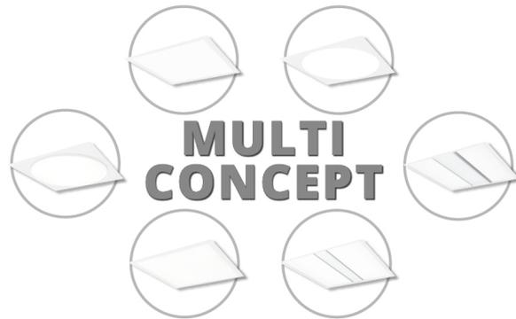
Multi Concept is a flexible, recessed luminaire that is designed to meet future requirements. The luminaire can be combined in a variety of ways using the three components (luminaire housing, insertable LED unit and front cover). Thus, Multi Concept is adaptable to a room's function in terms of design and lighting technology and the lighting can be optimised when the function of a room is changed.
