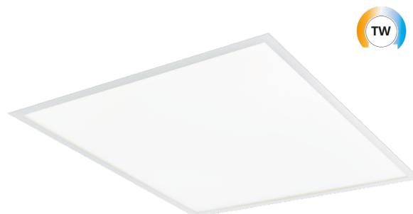
DiLED IV TW is a recessed mounted luminaire for most known ceiling systems in different modules. DiLED IV TW is suitable for office and general lighting indoor. The opal or prismatic optic front ensures a uniformly lit surface. Complete with driver and quick connection between driver and luminaire for super quick and easy mounting. Tunable White 2700-6500K DALI Type 8. Emergency box to be ordered separately.
