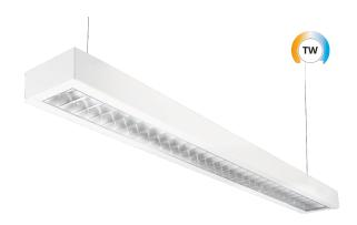
Flat design, powder-coated white RAL9010 gloss 25. Double parabolic reflector and diffuser with option of dimmable solution (DALI/SwitchDim). Plug-and-play solution for quick installation. Adjustable wire suspension (2x2 m) ordered as accessory. Tunable White from 2700 Kelvin to 6500 Kelvin white light. Controlled by Dali Type 8.
