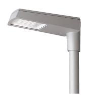
Design: Christian Hvidt. Mast top-mounted LED luminaire. IP66. LED luminaire. Base and top made of die-cast aluminium, front made of tempered glass. Base and diffuser in textured light grey. Direct lens optical solutions (Multilens). Complete with LED driver for operation of LED light sources mounted to component rail with internal connector/lampholder and pre-mounted with six-metre connection cable. Prepared for mounting on 60 mm mast. Safety class II.
