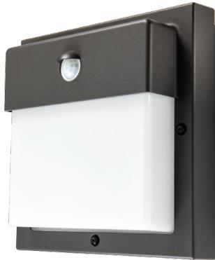
Attractive, square LED wall luminaire that can be installed both indoors and outdoors. Made of die-cast powder-coated aluminium. Diffuser made of UV-stabilised opalescent polycarbonate, two inputs/outputs for cables, option of both visible and hidden cabling, and loopable terminal block. IP65 and vandal-resistant rating IK10 with PIR sensor
