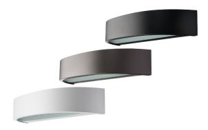
Round, attractive wall luminaire for horizontal/vertical installation and indoors/outdoors. Made of diecast powder-coated aluminium. Glass diffuser. Can be mounted as a downlight or as an uplight, IP65, integrated LED, mounting back panel with two inputs/outputs for cables, option of both visible and concealed cabling, and loopable quick clips. IP65 and vandal-resistant rating IK06.
