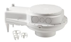
Concrete Box is used for embedding downlights. Tested and approved for SG downlights. Designed for rebar, solid PP in fire retardant V0 quality. Designed to provide a smooth casting process. Ø83 holes, for use with Junistar, Junistar ECO, Junistar Soft, and Uniled.
