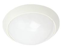
Round lamp in several sizes. Vandal-resistant with impact-resistant polycarbonate opalescent diffuser. The whole luminaire has been approved for common access routes and has vandal-resistant rating IK10. KI II, two cable inputs and the option of additional looping using the integrated quick clips. Can be mounted to either the wall or ceiling with both concealed and visible cabling. Many light source variants and sensors, wireless control and emergency light.
