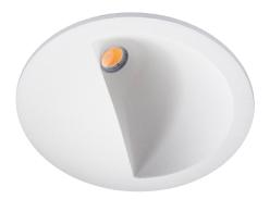
Attractive downlight for indoor use, particularly well suited to mirrors and effect lighting. Asymmetrical light curve, well integrated LED chip and associated dimmable driver. Made of die-cast powder-coated aluminium. 100-degre scattering angle. Low surface-mounted with Ø83 hole dimensions.
