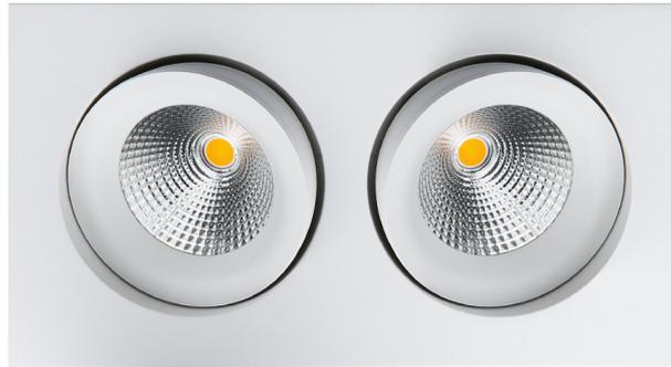
Attractive downlight for indoor use with 30-degree 360-degree stepless tilt. Well integrated LED chip and dimmable Phase cut-off. Made of die-cast powder-coated aluminium or brushed steel, glass diffuser. 42-degree scattering angle via reflector. Low recessed downlight with hole size Ø83mm. Tool-free mounting in mounting box for direct 230 V with loopable quick clips and automatic strain relief. IP44, KL III with dedicated circuit.
