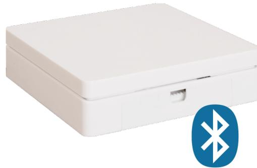
LEDDim Smart Floor is an indoor phasecut dimmer to be placed on the floor for connecting floor or table lamps - alternatively wall mount with slots on the back. The dimmer has a big button on top to On/Off or long push to regulate light level. Connect either a Europlug directly into it or connect, up to, 3 lamps via the terminals. It's possible to program without dimming and functioning as On/Off for lamps that requires this.
