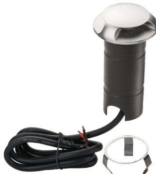
Luna Deco is a family of outdoor in-ground lights for effect lighting. They are perfect for lighting the edges of paths and other garden elements. They are also well suited for mounting in walls. They are made of acid-proof steel and powder coated machined aluminum. Totally waterproof, IP67. Has integrated, sealed LED light source. Comes with a tube for mounting in the ground, and with a clip for mounting in a wall. Delivered with cable for connecting to a 24V driver. 1-4 Luna Deco/Driver.
