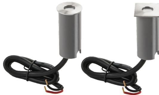
Luna Mini is an in-ground light perfectly suited for surrounding pools and other stylish environments. It is also well suited for mounting in walls. Both a round and a square front is included to fit every taste. It is made of acid-proof steel and powder coated machined aluminum. Totally waterproof, IP67. It has integrated, sealed LED light source. Comes with a tube for mounting in the ground, and with a clip for mounting in a wall. Delivered with cable for connecting to a 24V driver.
