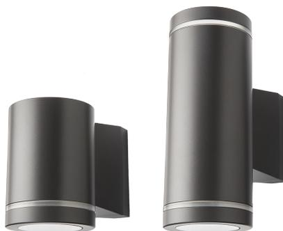
Round wall luminaire for outdoor installation. Available both as an upward/downward light and as a downward light. The luminaire has an interchangeable GU10 LED light source (included) and is dimmable with a trailing-edge dimmer. Simple installation with a wall bracket and connector for the lamp, two cable inputs and the option of both visible and concealed cabling. Can be mounted on a corner with a corner bracket (sold separately).
