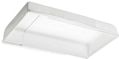
Pull-out Multibox, adjustable from 33-60 cm. Suitable for Junistar and Capella. Attached with double-sided tape for mounting of diffusion plate. Mounting of K-tube is done without the use of cupboard sleeve or clips. Manufactured from recycled, heat-resistant, halogen-free, and flame-retardant (V0) material. L: 330-600 mm B: 280 mm H: 65 mm
