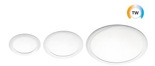
Sense luminaire used as replacement or alternative for a normal downlight. Very low profile and quick connection between luminaire and driver as well as tool-free connection in junction box with loop for easy and quick installation. High efficiency up to 105 lm/W and low glare rating makes Sense the obvious choise in many applications. Tunable White 2700-6500K LEDDim or DALI Type 8.
