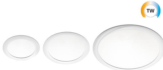
Sense luminaire used as replacement or alternative for a normal downlight. Very low profile and quick connection between luminaire and driver as well as tool-free connection in junction box with loop for easy and quick installation. High efficiency up to 105 lm/W and low glare rating makes Sense the obvious choice in many applications. Tunable White 2700-6500K LEDDim or DALI Type 8.
