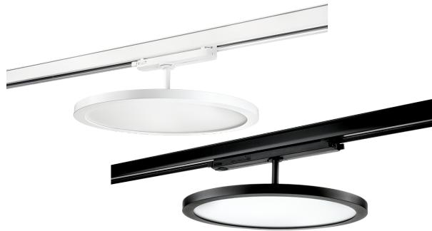
General lighting luminaire for ShopLine three-phase track systems. It can even be used with other track systems that fits Global adapters. Stylish, thin disc, with opal prismatic front, directing the light and securing low glare. The driver is integrated in the track adapter.
