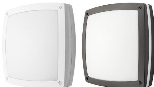
Attractive, square luminaire with direct and indirect light that can be mounted to both walls and ceilings, and both indoors and outdoors. Made of die-cast powder-coated aluminium. Flat diffuser with indirect light made of UV-stabilised opal polycarbonate. Several light source variants and sensors, and wireless control. Two inputs/outputs for cables, option of both visible and concealed cabling, and loopable terminal block. IP65 and vandal-resistant rating IK10.
