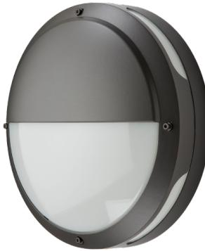
Design: Svein Knudsen / Andrew Smith. Attractive, round wall luminaire with half-diffuser and four slits for indirect light that can be installed both indoors and outdoors. Made of die-cast powder-coated aluminium. Diffuser made of UV-stabilised opal polycarbonate. Two inputs/outputs for cables, option of both visible and concealed cabling, and loopable quick clips. IP65 and vandal-resistant rating IK10.
