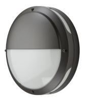
Design: Svein Knudsen / Andrew Smith. Attractive, round wall luminaire with half-diffuser and four slits for indirect light that can be installed both indoors and outdoors. Made of die-cast powder-coated aluminium. Diffuser made of UV-stabilised opal polycarbonate. Two inputs/outputs for cables, option of both visible and concealed cabling, and loopable quick clips. IP65 and vandal-resistant rating IK10.
