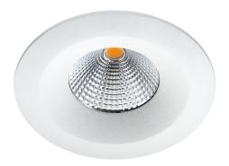
Attractive downlight for indoor and outdoor use. Mounted directly in the insulation. Well integrated LED chip, dimmable via phase-dimming or DALI driver (not IsoSafe). Made of die-cast powder-coated aluminium or brushed steel (only indoors), glass diffuser. 42-degree scattering angle via reflector. 35 mm in total height, Flexible hole dimensions Ø76–Ø83. Tool-free mounting in mounting box for direct 230 V with loopable quick clips and automatic strain relief. IP54, Class II
