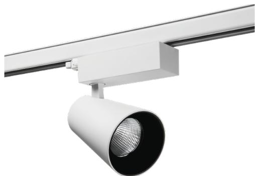
LED spot for three-phase rail system. Fitted with global adapter and compatible with all systems that work with this. Powerful LED chip and integrated driver gives this spot a minimalistic and exclusive look. Luminaire body made of powder-coated aluminium, 50-degree reflector that can be replaced with 17 or 32-degree reflector. A long service life, fantastic colour retention and large lumen package make Vision the ideal choice for shops and exhibitions.
