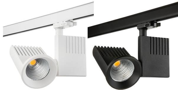
Three-phase rail spot with integrated powerful LED chip and driver. Driver can switch between three brightness levels using a jumper terminal. Mounted using global multi-adapter, which is ideal for SG's three-phase rail system (Shopline) as well as other systems where Global can be used. ZIP is made of powder-coated aluminium, flexible and able to be pointed in almost all directions, making it the obvious choice for shops and exhibitions.
