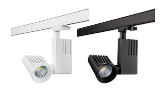
Three-phase rail spot with integrated powerful LED chip and driver. Dimmable with phase dimmer. Mounted using global multi-adapter, which is ideal for SG's three-phase rail system as well as other systems where Global can be used. Perfect colour rendering due to very high RA value and SDCM 2. ZIP Pro Mini is made of powder-coated aluminium, flexible and able to be pointed in almost all directions, making it the obvious choice for all places where spots or effect lighting is to be used.
