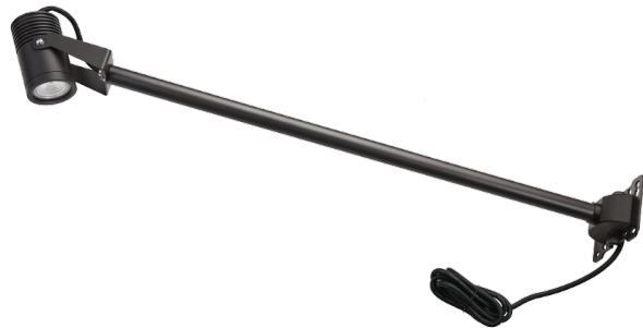
Hovden Sign is a signboard luminaire for outdoor use featuring a flexible luminaire head that can be turned towards wherever light is needed. Manufactured from powder-coated aluminium. Supplied with a 1-metre cable with free end. Dimmable using phase control. It includes an integrated, sealed light source which means the luminaire is IP67 waterproof. Additional glare covers are available as accessories.
