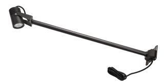
Hovden Sign is a signboard luminaire for outdoor use featuring a flexible luminaire head that can be turned towards wherever light is needed. Manufactured from powder-coated aluminium. Supplied with a 1-metre cable with free end. Dimmable using phase control. It includes an integrated, sealed light source which means the luminaire is IP67 waterproof. Additional glare covers are available as accessories.
