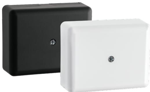
Junction box for wall mounting, IP20. Supplied with 6 removable screw terminals for up to 2x6mm<sup>2</sup>. Recesses in corners and sides of the box. Option for 16mm pipe entry at the bottom. Manufactured in colour-fast polycarbonate.
