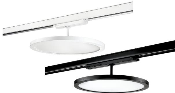
General lighting luminaire for ShopLine DALI three-phase track systems. It can even be used with other track systems that fits Global DALI adapters. Stylish, thin disc, with opal prismatic front, directing the light and securing low glare. The driver is Integrated in the track adapter.
