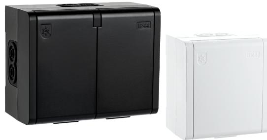
IP44 outlet for outdoor and indoor use, in laundry rooms, and similar areas. Available in white and black, single and double outlets with child protection, and flip covers with automatic locking. Cable bushings in soft polymer, the cable bushings are moved and, if needed, replaced by a strain relief (accessory). There are also weak points for cable entry from behind, making it IP44, and weak points for drainage must be opened.
