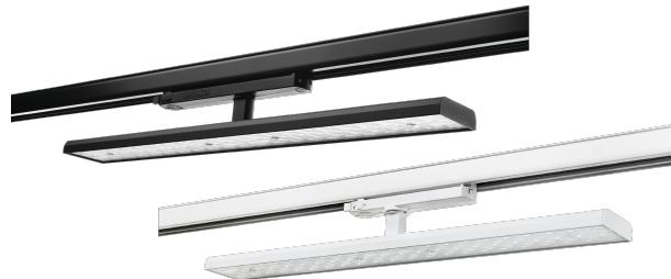
Luminaire for general lighting for the ShopLine three-phase track system. Can also be used with other track systems that utilize Global. Stylish, slim fixture with lens technology that directs the light where it's needed. The driver is integrated into the track adapter and includes dip switches, facilitating adjustment of light output or reduced UGR.
