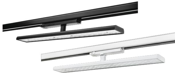
Luminaire for general lighting for the ShopLine DALI three-phase track system. Can also be used with other track systems that fits Global DALI adapters. Stylish, slim fixture with lens technology that directs the light where it's needed. The driver is integrated into the track adapter and includes dip switches, facilitating adjustment of light output or reduced UGR.
