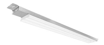
Efficient industrial luminaire, mounted directly on ceiling or suspended on wire. Cable connection at the ends with  $5 \times 2.5$  mm prewiring. Made of galvanised steel with powder-coated white reflector and opal diffuser
