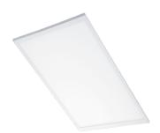
The Sense Basic 300x600 LED panel is ideal both for new installations and remodelling projects. It can directly replace 2x14W T5 and 2x18W T8 luminaires. It has a lightweight steel housing and is based on backlight, yet it is only 35 mm height. High quality non-yellowing PMMA micro prismatic front optics. Easy tool-free installation, twist connector between driver and panel and junction box with automatic strain relief for cables or plastic tubing.
