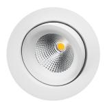
Attractive downlight for indoor use with 30-degree 360-degree stepless tilt. Well integrated LED chip and dimmable Phase cut-off or DALI driver. Made of die-cast powder-coated aluminium or brushed steel, glass diffuser. 42-degree beam angle angle via reflector. Low recessed downlight with hole size Ø83mm. Tool-free mounting in mounting box for direct 230V with loopable quick clips and automatic strain relief. IP44, KL III with dedicated circuit.
