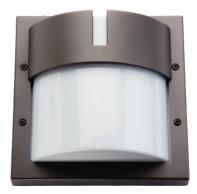
Square wall luminaire with half diffuser and slit for indirect light. Extra protection of diffuser. Made of die-cast powder-coated aluminium. Diffuser made of UV-stabilised opal polycarbonate. Two inputs/outputs for cables, option of both visible and concealed cabling, and loopable quick clips. IP65 and vandal-resistant rating IK10.
